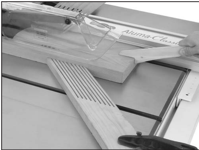
Figure 60. Typical ripping operation.
